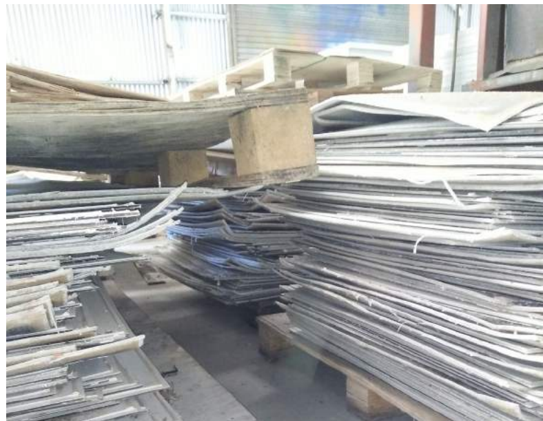
Failed solar panels in recycling yard. (Frames already removed).
